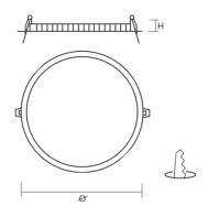
M1: Ø225 mm H:12mm Hueco= Ø200mm M2: Ø 290mm H: 12mm Hueco= Ø280 mm
